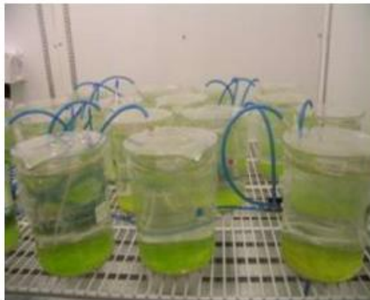
Figure 4. The test for the inhibition of growth on microalgae or cyanobacteria is the quantified measurement of toxic effects of chemical substances (pollutants) on primary producers in freshwater or marine ecosystems.
