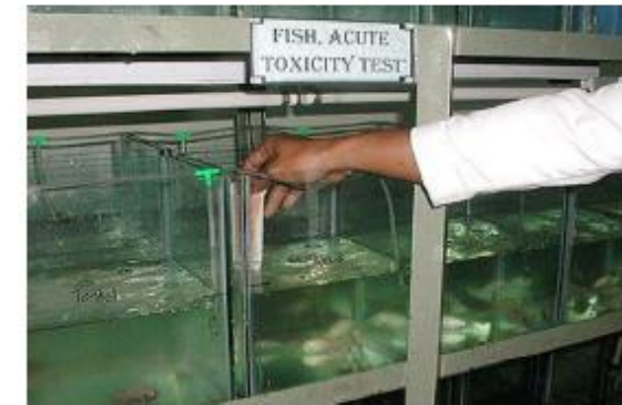
Figure 6. The acute toxicity test in fish is normally for the duration of 4 days (96 hrs) with the toxic substance administered in at least 5 concentrations. The cumulative % mortality is plotted against \log concentration and the LD_{50} or LC_{50} is estimated from the concentration-response curve.
