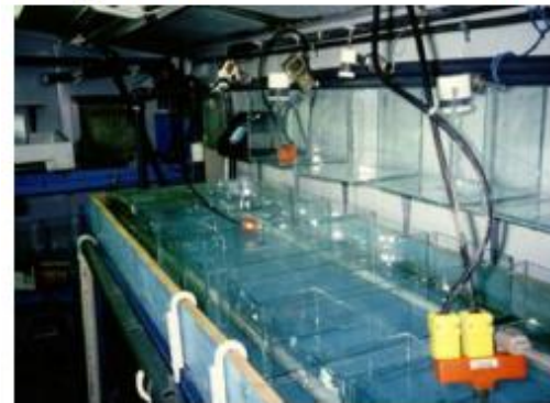
Figure 6. The acute toxicity test in fish is normally for the duration of 4 days (96 hrs) with the toxic substance administered in at least 5 concentrations. The cumulative % mortality is plotted against \log concentration and the LD_{50} or LC_{50} is estimated from the concentration-response curve.
